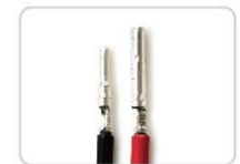
Use crimping pliers to fix-copper terminals on the end of stripped cable.
